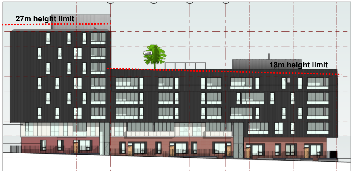
Figure 51 – Proposed Building C (western, Leticia Street elevation) demonstrating breach of 18m height control (from new public domain ground floor level)
