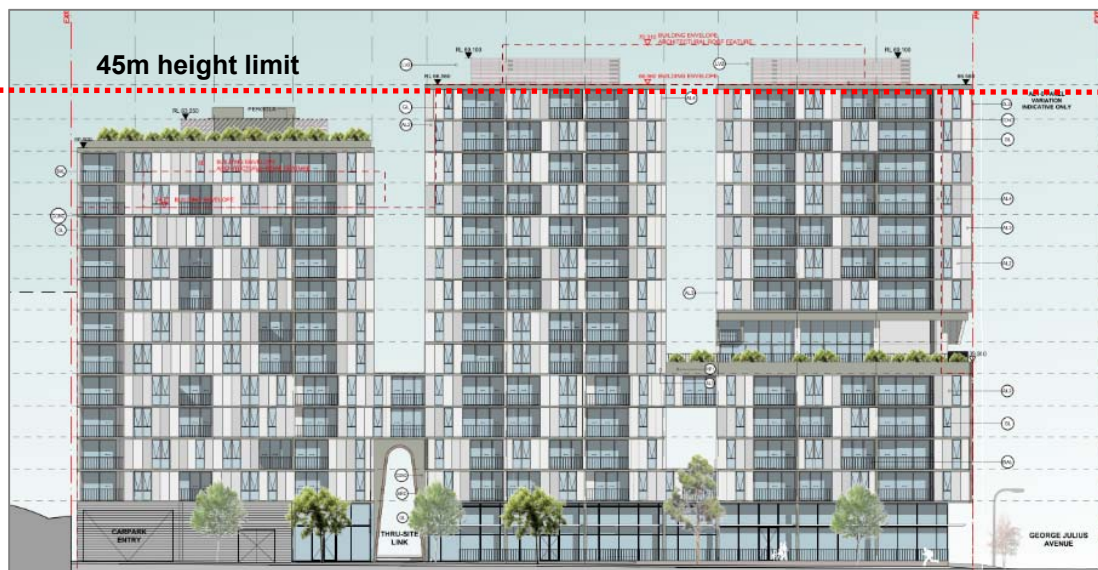
Figure 45 – Proposed Building A demonstrating breach of 45m height control (from new public domain ground floor level)
