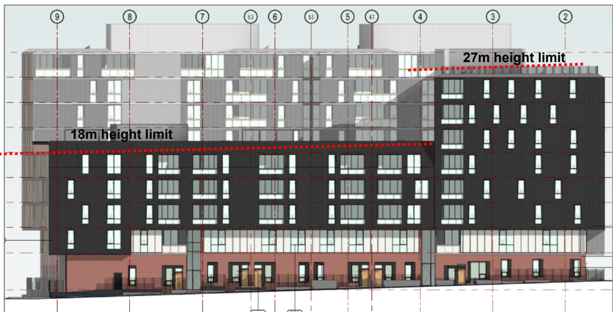
Figure 48 – Proposed Building B (eastern, Leticia Street elevation) demonstrating breach of 18m height control (from new public domain ground floor level)
