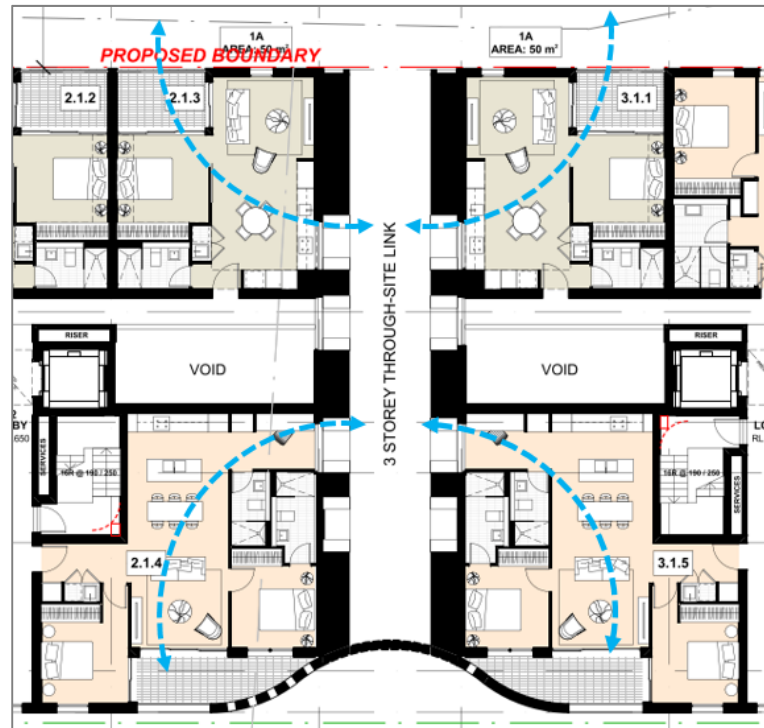
Figure 57 – Building A Level 2 and 3 - windows to through site link required for natural cross ventilation
