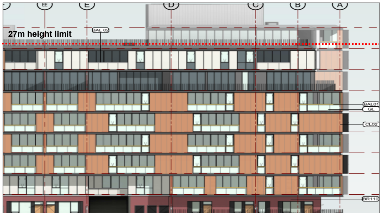
Figure 46 – Proposed Building B (northern, Peters Street elevation) demonstrating breach of 27m height control (from new public domain ground floor level)
