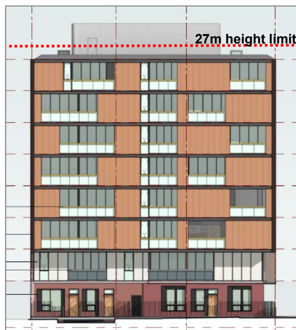
Figure 50 – Proposed Building C (northern, Peters Street elevation) demonstrating breach of 27m height control (from new public domain ground floor level)
