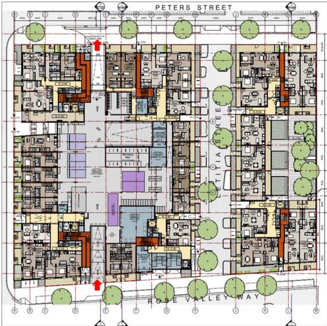
Figure 37: Access and egress through ground floor parking area to Building B
